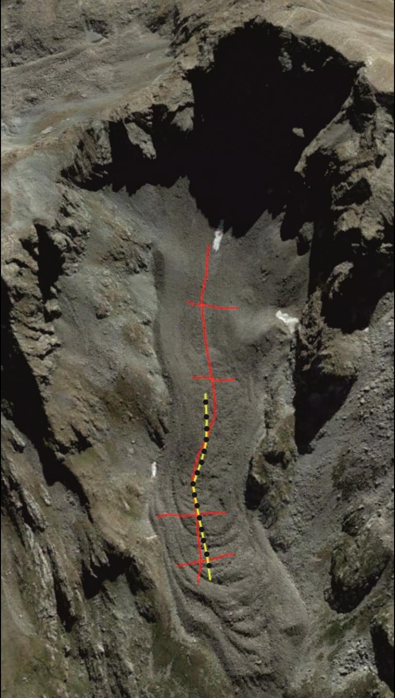
Red lines: Ground-Penetrating Radar profiles Yellow line: Electrical Resistivity Tomography profile Yellow line is 260 m long
